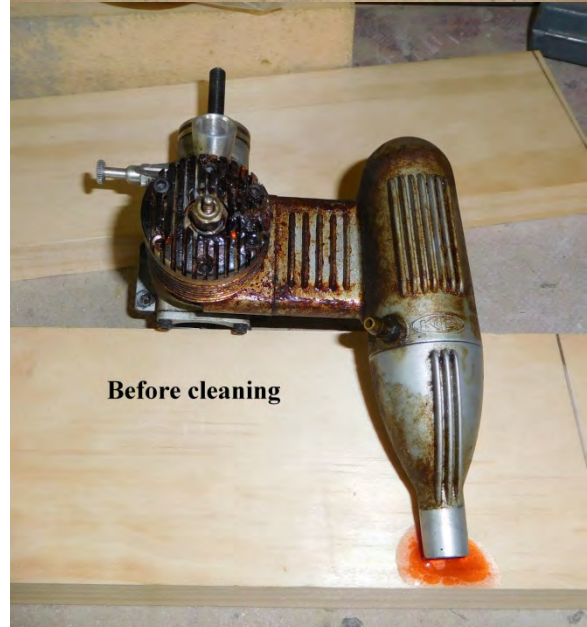
Winter oil leaking from muffler. I use Marvel air tool oil.
