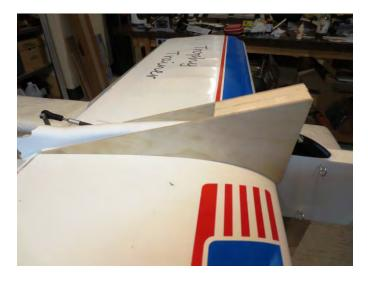
It's a two sided ramp that fits over the fuselage front to form a ramp to guide the cut.
