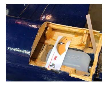
I braced up the broken and cut bulkheads, added a half bulk head over the tank, and reinforced the forward area to brace the sheet balsa. Then I cut off the antenna, and rerouted the fill line to the inside in the unfortunate case of an inverted landing.
