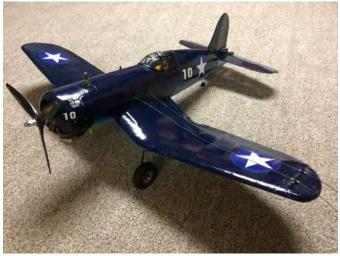
You may have read in the October flying reports, we found that the Corsair had the unfortunate characteristic of running fuel out the inverted venturi while at rest, and fuel-locking the engine. After some fiddling, it was retired from the flight line for repairs.
