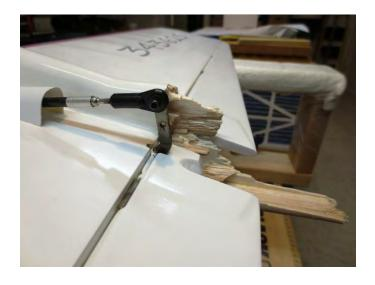
The Trophy Trainer sat all summer while I tried to figure out how to repair it. Obviously a new fuselage section would have to be made, but how do I attach it to the wing and how do I clean up the damage to form a good glue line and maintain alignment? I thought of several ways I could make a whole lot of work for myself until I thought of this:
