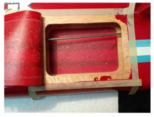
I needed to protect the plane from catching fire, so lined the cavity with Aluminum foil and wet paper towels. Then used a Dremel to cut the Music Wire. A split roll pin was used to join the two pieces of Music Wire back together. Hammered on the split roll pin to make a tight fit with the Music Wire, so it would stay in place when soldered together.
