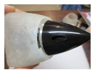
From the backside showing the firewall to be glued into the fuselage:
