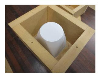
Filled it with silicone rubber and made the mold:
