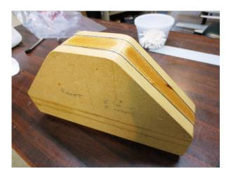
The dark lines on the previous picture are string CA'd to the mold to mark the cut outline.
