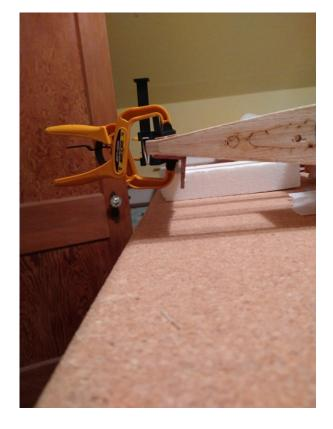
A little bit of overkill here. I added an aluminum angle iron to the top. To ensure that both sides are as straight as they can be. Maybe the wood will learn to stay that way when I remove the clamps.
